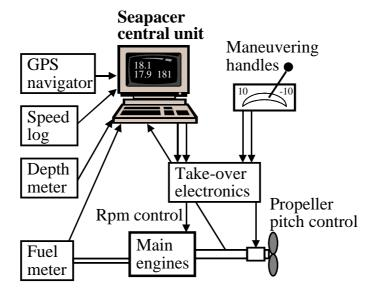
Figure 2: Block diagram of a basic system. The central unit takes over control from the maneuvering handles and controls the main engine speed and propeller pitch.
