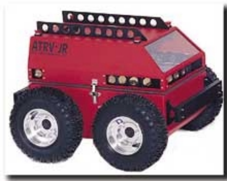
Figure 3. The ATRV-JR from iRobot. HxL: 55cm x 77.5cm. Weight: 50kg. Photo courtesy of iRobot Corporation.
