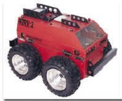
Figure 2. The ATRV from iRobot. HxL:65cm x 105cm. Weight: 118kg. Photo courtesy of iRobot Corporation.
