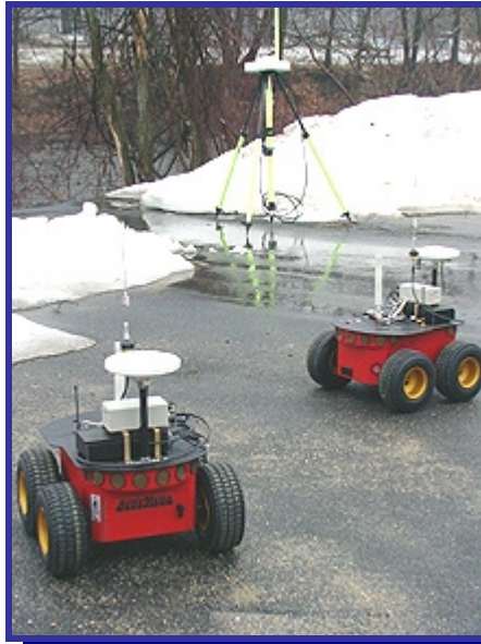
Figure 4. Pioneer 2-AT from ActiveMedia Robotics. HxLxW: 26cm x 50cm x 49cm. Weight: 30kg. . Photo courtesy of ActivMedia Robotics.
