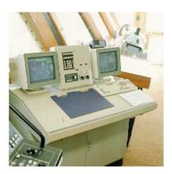
Figure 1: The central unit placed on the bridge of the vessel. The left screen is used for real-time control tasks such as speed settings while the right screen is used for long term voyage analysis and follow-up.
