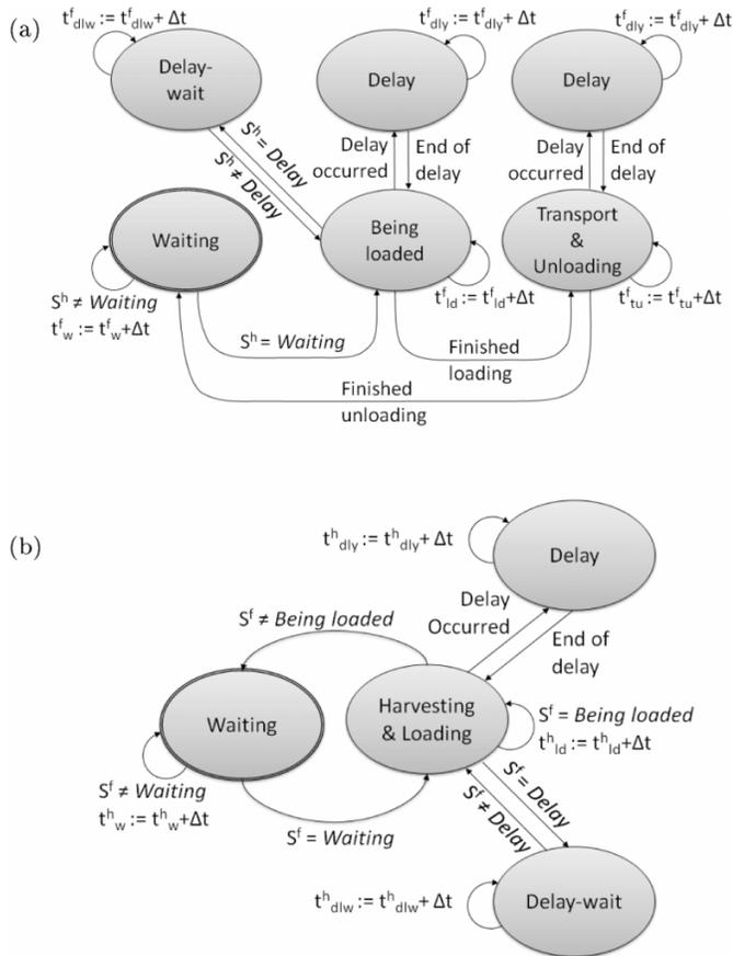
**Fig. 3.** State diagram for one or more autonomous forwarders changing loads with a harwarder (ALC system).  $S^h$  and  $S^f$  are the current states of the harwarder and forwarder, respectively. Time  $t$  is incremented by  $\Delta t$  in each simulator step. At the start of each simulation, the harwarder is initialized to state “Harvesting & Loading” and the forwarder to state Waiting. (a) Load-changing forwarder. (b) Load-changing harwarder.
