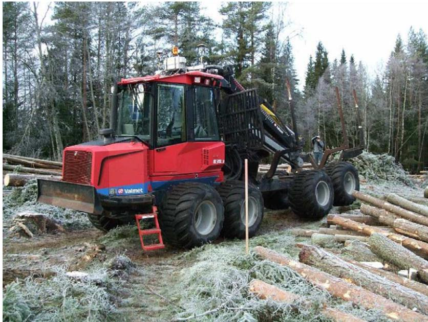
Figure 1. The studied Valmet 830 forwarder equipped with an RTK DGPS for localization and heading measurements and a gyro determining the vehicle's roll and pitch angles.
