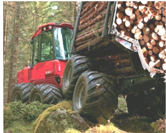
Fig. 2. Bogie negotiating a stone and reducing the obstacle height. Photo courtesy of Komatsu Forest AB.
