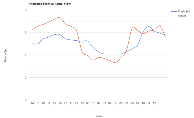
Fig. 7. Predicted flow rate based on data from non-flow sensors vs. actual flow rate.
