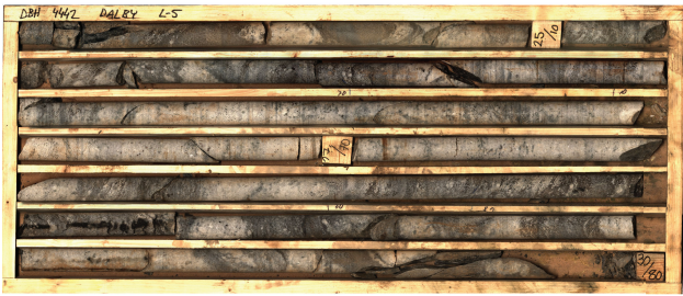
Fig. 1. Example optical photograph of a core box with rock samples. Notice the heterogeneity of rock types.
