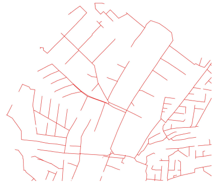
Fig. 3. Sewage water pipe system in Näsby.
