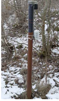
Fig. 4. A ground water level sensor with wireless communication.
