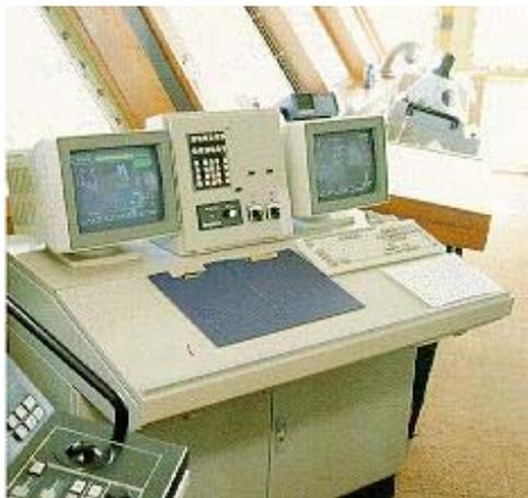
Figure 1: The central unit placed on the bridge of the vessel. The left screen is used for real-time control tasks such as speed settings while the right screen is used for long term voyage analysis and follow-up.
