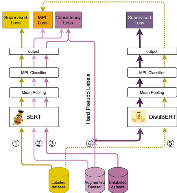
**Figure 2: The teacher(left network)-student(right network) architecture of Distill-*Cformer*.**
