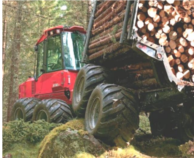
Figure 2. Bogie negotiating a stone and reducing the obstacle height. Photo courtesy of Komatsu Forest AB.
