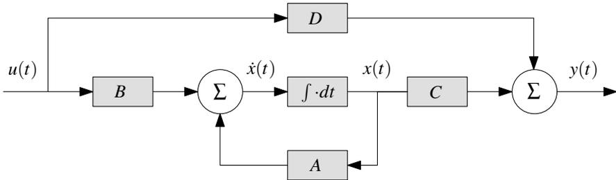
FIGURE 2.2: Block diagram of a linear time-invariant system in continuous time.
