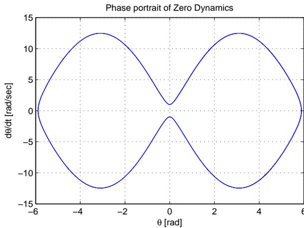
FIGURE 5.4: Phase portrait of a periodic trajectory of the Furuta pendulum, where  $\theta$  is the angle of the pendulum.
