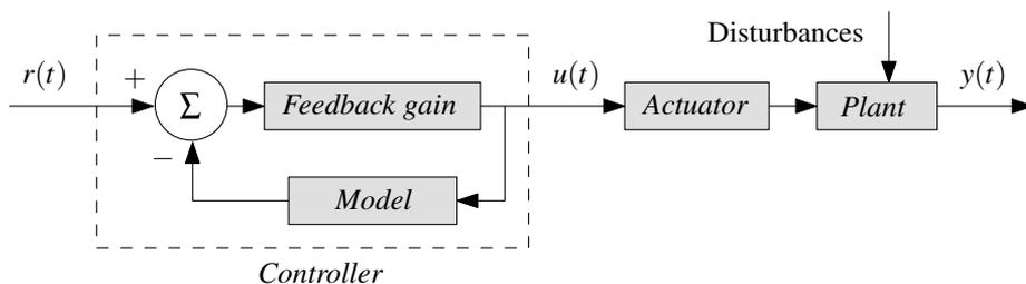
FIGURE 3.2: Open-loop system.
