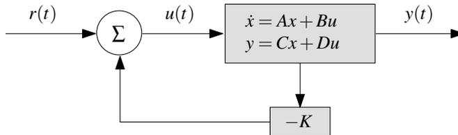
FIGURE 3.4: State-feedback controller.
