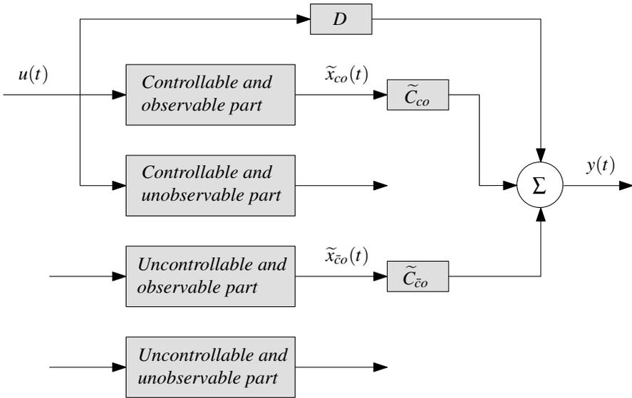
FIGURE 2.5: Block diagram of the Kalman canonical decomposition.
