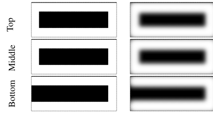
Fig. 4. Initial design variables and its corresponding filtered designs over the three-layer design domain, arranged from bottom to top.
