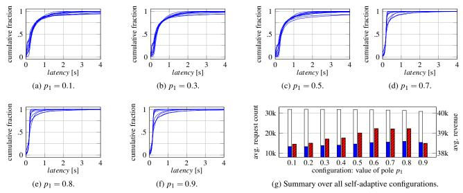
Figure 6: Statistical results for self-adaptive system. Figs. 6a to 6f show empirical cumulative distribution of latencies for each configuration. Each line represents the results of a test-case. Fig. 6g shows, for each configuration, over all test-cases, average served requests in total (bar with no fill) and with recommendations (solid, blue bar), and average revenue (red, patterned bar).
