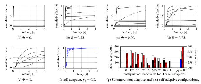
Figure 7: Statistical results for non-adaptive system. Figs. 7a to 7e show latency distribution for each non-adaptive configuration, while Fig. 7f shows our selected self-adaptive behavior. Each line represents a test-case. Fig. 6g shows, for each configuration, over all test-cases, served requests in total (bar with no fill) and with recommendations (solid bar), and revenue (red, patterned bar).
