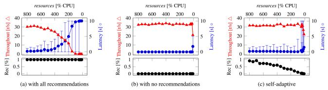
Figure 1: Stress-testing RUBiS extended with our recommender engine. The number of users is kept constant and the amount of CPU allocated is reduced. Throughput reduction and response time increase show the point where the application is saturated.
