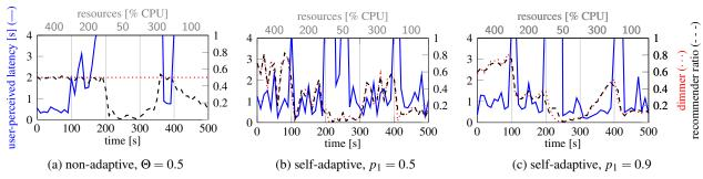
Figure 3: RUBiS behavior in a non-adaptive configuration and two self-adaptive configurations, varying the resource allocation.
