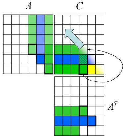
**Fig. 2.** The symmetric LYCT wavefront: standard, one-sided, symmetric. Each subsolution (i.e., a block of the solution matrix  $X$ ) located outside the main block anti-diagonal is broadcasted in the corresponding block row and column and the block row corresponding to its transposed position.
